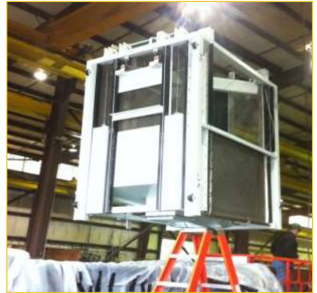
Fabricated Fish Hopper
