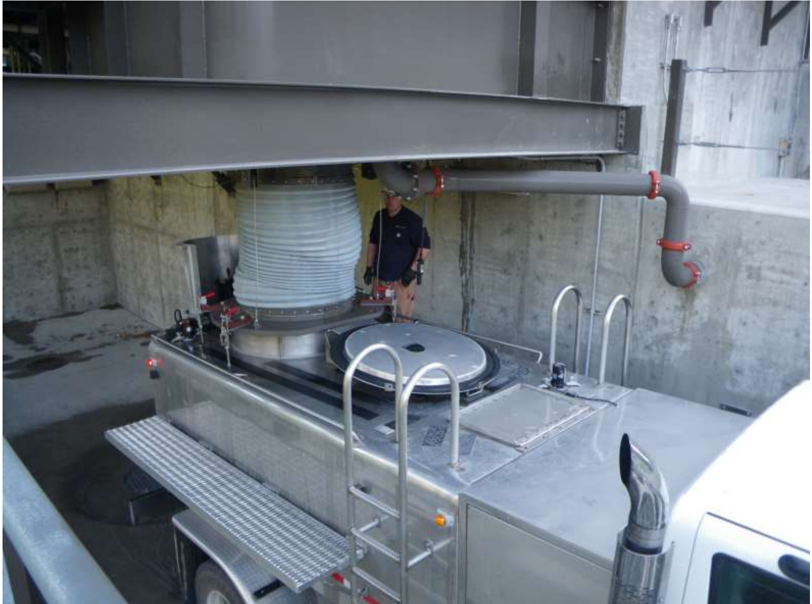
Fish Crowded to Loading Tank above for Water-to-Water Truck Loading
